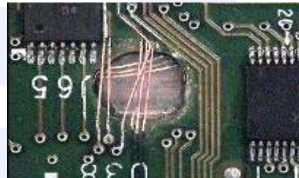
Inner Trace Repair
